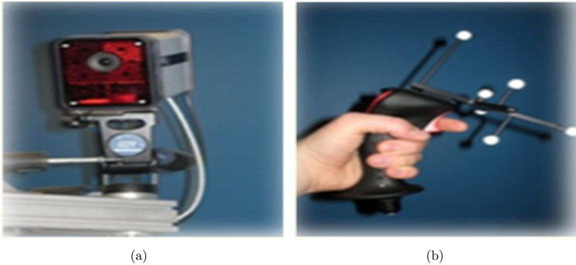
Figure 5.16: Tracking system of the semi-immersive platform (a) Infrared camera ;(b) Flystick with shining balls
