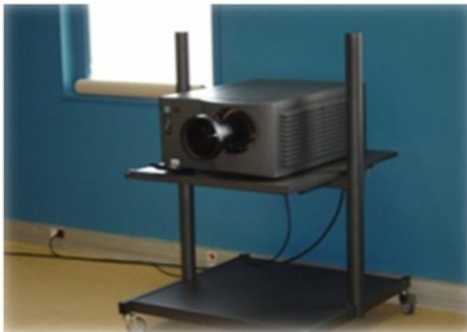
Figure 5.15: The DLP Mirage 4000 projector of the evr@ platform.
