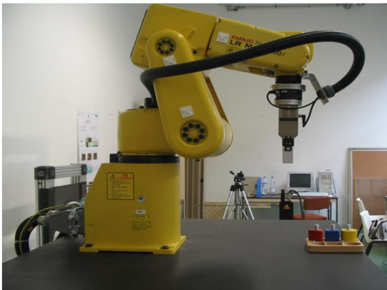
Figure 5.20: Robot Fanuc LR MATE 200i.
