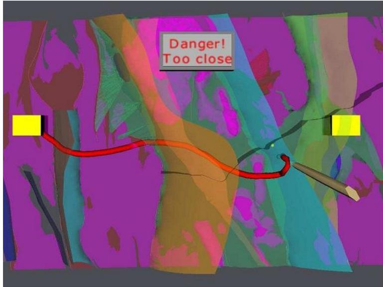
Figure 1.15: Screenshot of mine planning stage, showing geological layers of rocks and road tunnel
